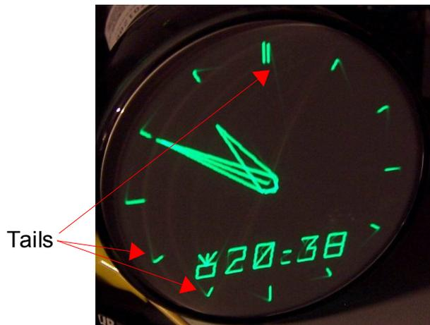
*The photo shows an optimum adjustment of brightness, focus and astigmatism.*
